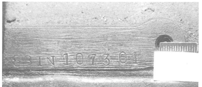
FIG. 6—Cylinder head showing the engine number and deep filing marks.
