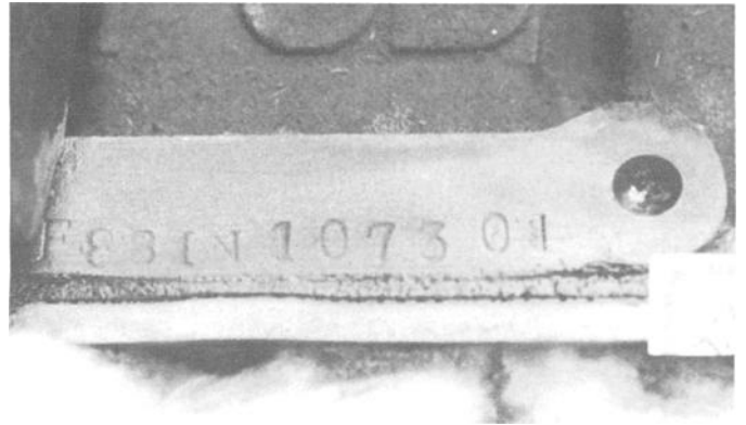
FIG. 5—Surface bearing the punched (Engine) number on the cylinder head.
