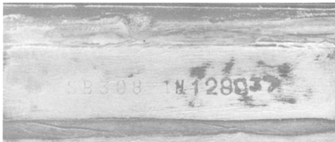
FIG. 4—Punched numbers on the chassis beneath the metal piece (Fig. 3) separated from the chassis.
