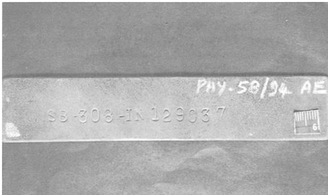
FIG. 3—The tailor-made iron metal piece bearing the present number “SB 308 IN 128037” separated from the chassis.
