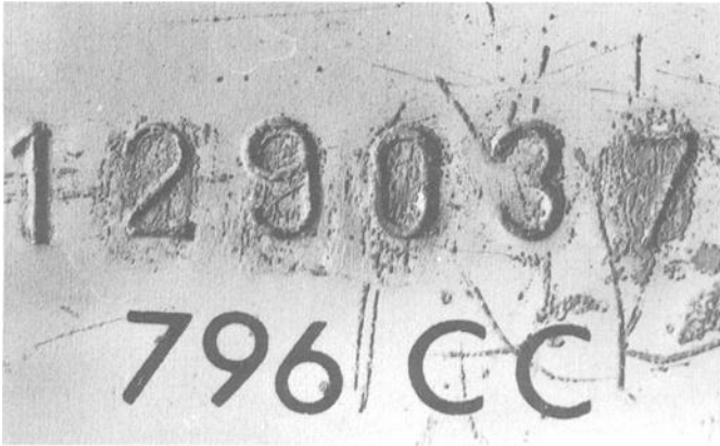
FIG. 8—Photograph showing the superficial erasure and the erased chassis number (see Fig. 7).
