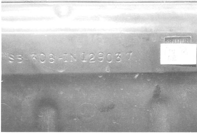
FIG. 2—The present chassis number on the chassis.
